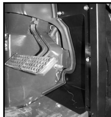
**x)** Installing the two side panels will take two people and a bit of finesse. The back and front edges of side panels need to be tucked behind the back panel fig.16 *cross section* and then the front panel fig.17 *cross section*. Install all fasteners see fig.6.
