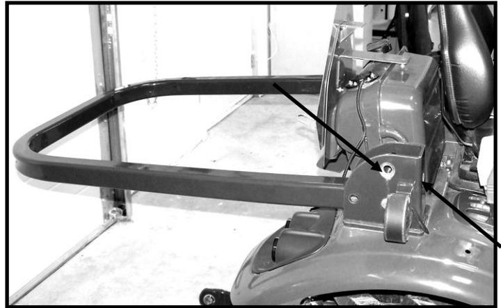
iii) Remove the side grab handle .You will also need to remove rubber floor mats. On the left hand side you will need to remove the plastic cover for front loader controls to remove the floor mat.
