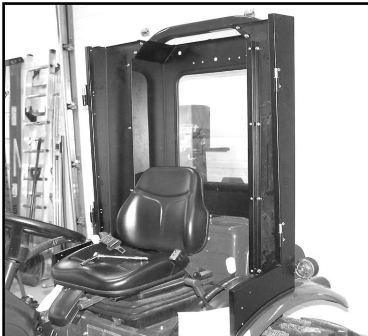
**ix)** Run 5/8" bulb molding provided along hood profile edge on the front panel fig.10 and along the two foot spacer box fig.11. Drop front panel on tractor fig.12. Attach Foot spacer boxes with 1/2", 1/4-20 SS Button head, and serrated flanged nut fig.13/fig.14. Leave both fasteners for bottom holes on foot spacer empty until side panels are put on. 3/4", 1/4-20 SS Button head are provided for the bottom holes.
