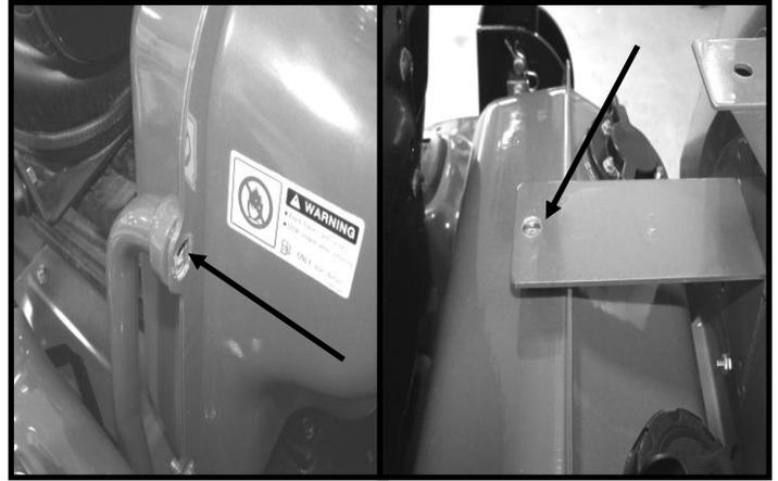
ii) Remove ROPS pins. Lower the ROPS and remove the two Left and right adjustment stoppers. This will allow room to install the back panel. The two adjustment stoppers will be used later to attach the left and right rear corner panels.
