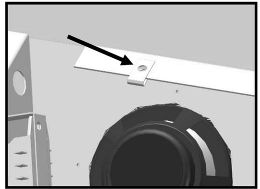
**ii)** The console drops on top of the cab before dropping the roof fig.2. The front lip sits on top of the front panel and the sides on top of the side panels.
