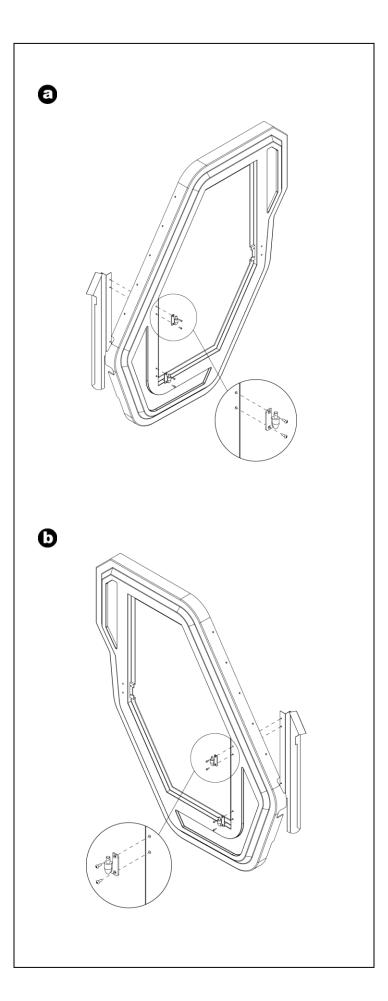
c) Install both hinge halves on driver side door using four (4) 10-32 x 1/2" screws, two (2) adjustment plates and one 1/4"-20 heavy duty lock nut. Insert (1) 1/4" Flat Washer between door and hinge as shown by arrow. Ensure hinges are oriented as shown in figure to the right.
