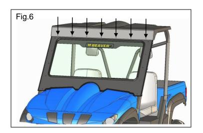
vii) Fasten roof panel to windshield panel using (7) ½-20 x 3/4" screws, washers and nyloc nuts (Fig.7).
